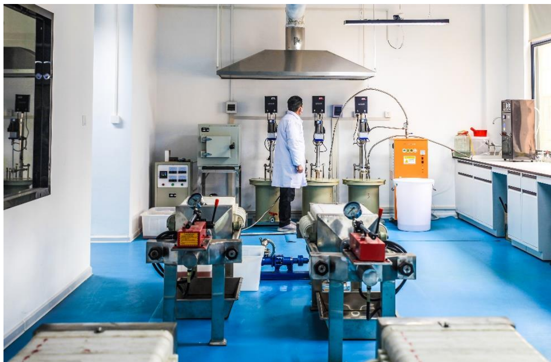
Image 6: Filter press (foreground) and sulphate reactors (background)
