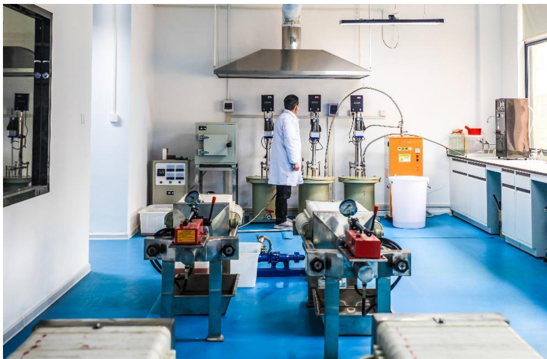
Image 6: Filter press (foreground) and sulphate reactors (background)
