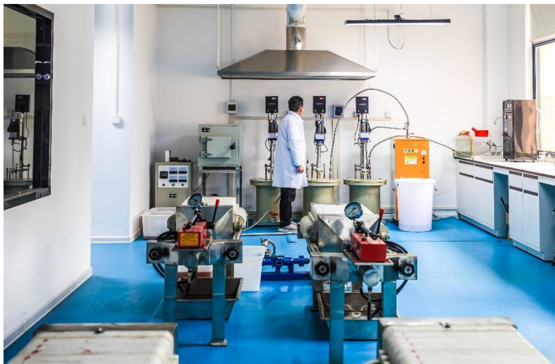
Image 6: Filter press (foreground) and sulphate reactors (background)
