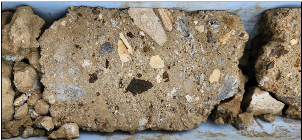
Figure 15. MLIDD020_178.0m_Polymictic Breccia with silica-pyrite clast
