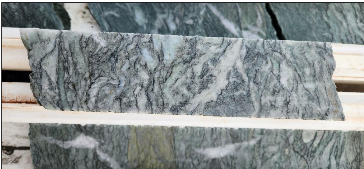
Figure 19. MLJDD019_148.4m_visceral texture in bleached, silicified ultramafic.
