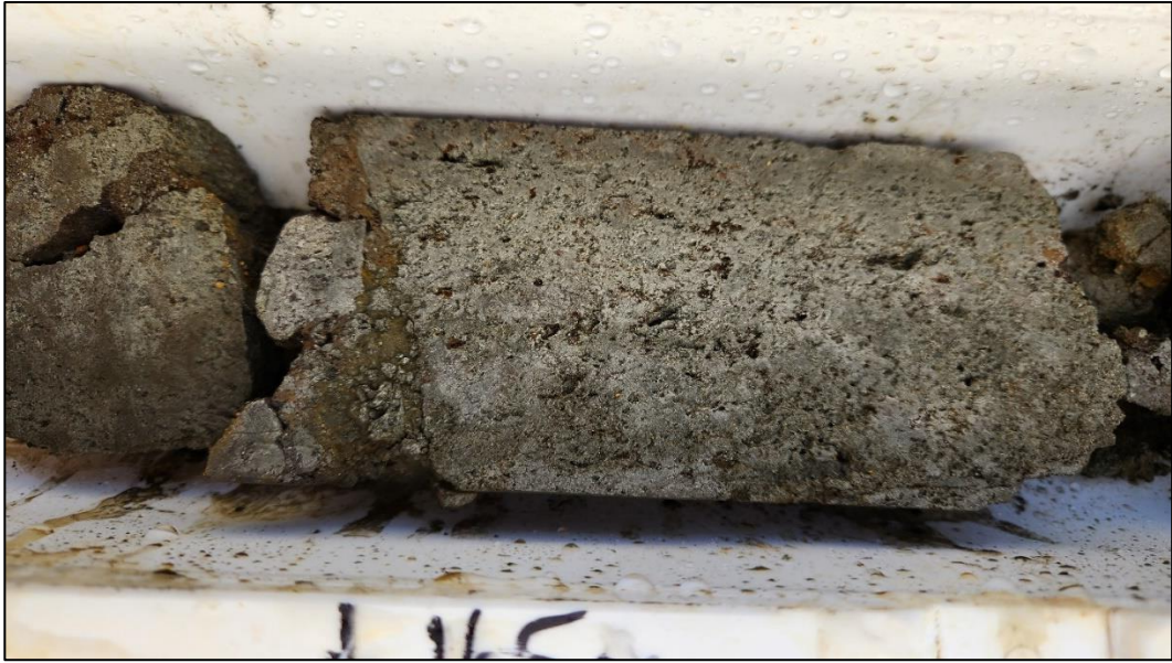
Figure 17. MLJDD018_164.5m_Massive pyrite in Breccia
