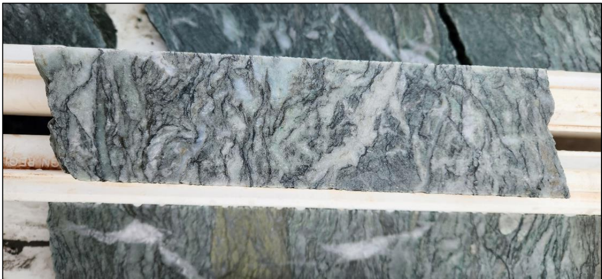
Figure 19. MLJDD019_148.4m_visceral texture in bleached, silicified ultramafic.
