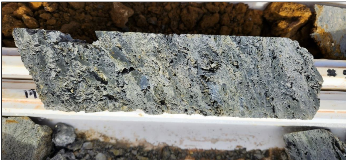
Figure 18. MLJDD018_198.0m Vuggy Silica Alteration
