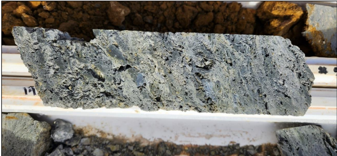
Figure 18. MLJDD018_198.0m Vuggy Silica Alteration
