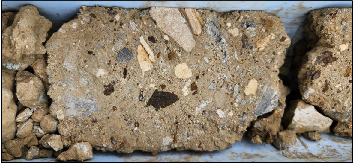
Figure 15. MLIDD020_178.0m_Polymictic Breccia with silica-pyrite clast
