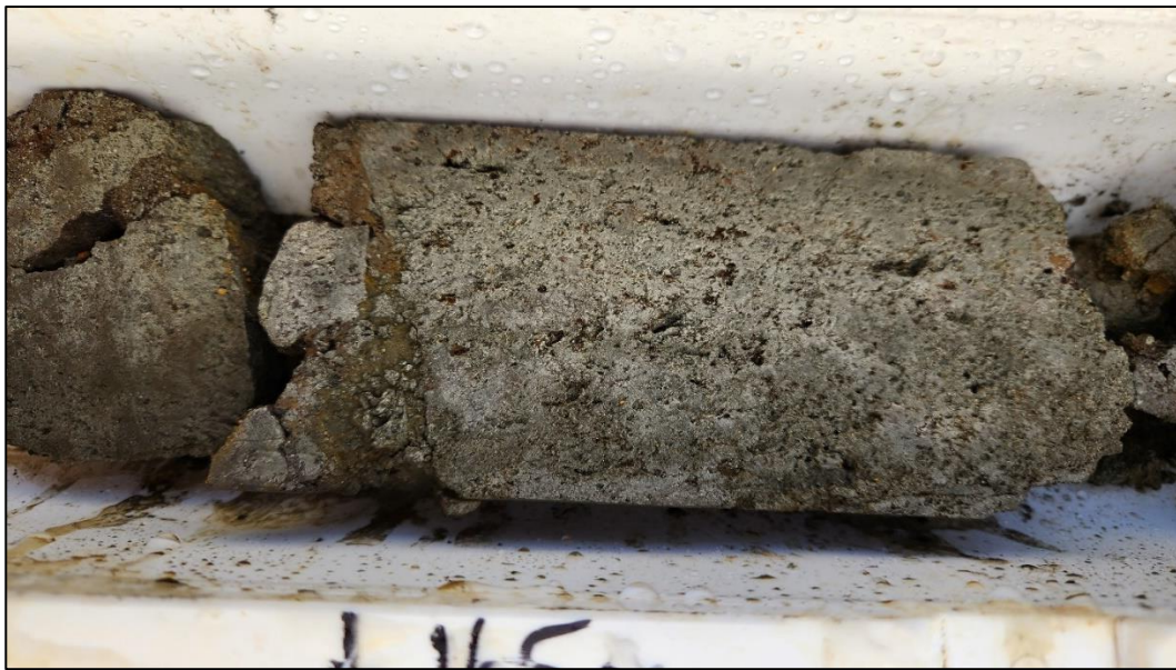
Figure 17. MLJDD018_164.5m_Massive pyrite in Breccia
