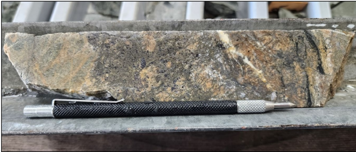
Figure 13 - 2019FTD007E, 129.8m - Mineralised carbonate-pyrite-arsenopyrite-cobaltite-scheelite vein (Interval 129.5-130.0m Assay: 0.5m @ 6.64g/t Au, 0.38% Co, 1.02% WO 3 , 0.11% Cu).
