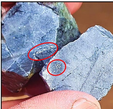
Figure 3: visible gold in cut samples at 123 to 124m interval (above) and sulphide mineralisation in sediments (right) at 123.4m drill depth
