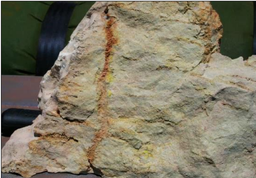
Figure 1: Carnotite (uranium) mineralisation (yellow mineral) in porous sandy limestone from the Ben Hur prospect. 2
