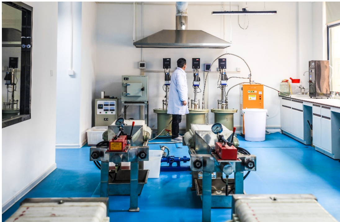
Image 2: Filter press (foreground) and sulphate reactors (background)
