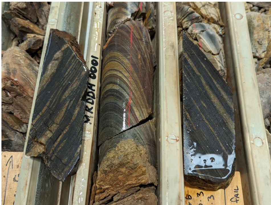
Figure 5. Comparison of magnetite-rich banded iron formation from the Cleaverville Formation (centre) with samples from historic Whaleshark diamond drill holes (left and right).
