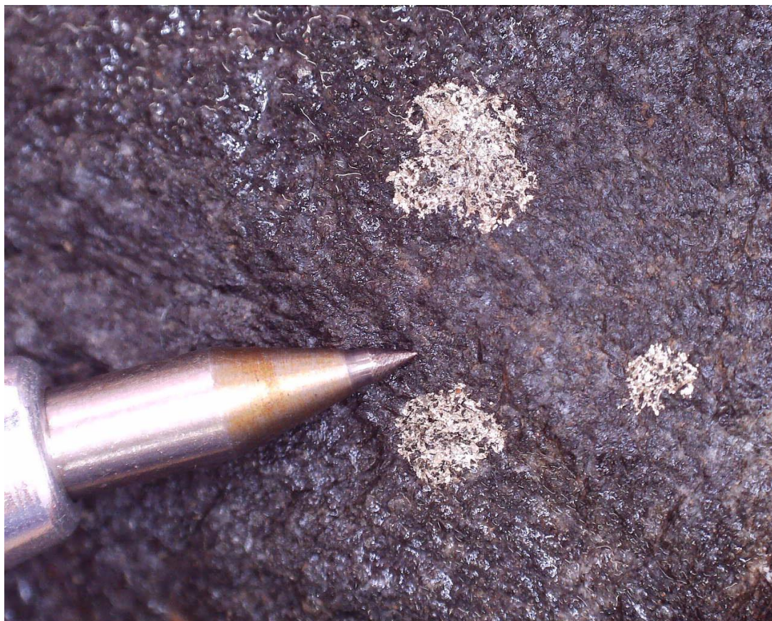
Figure 12. Coarse-grained pyrite “clots” in fine grained dolerite chill margin.
