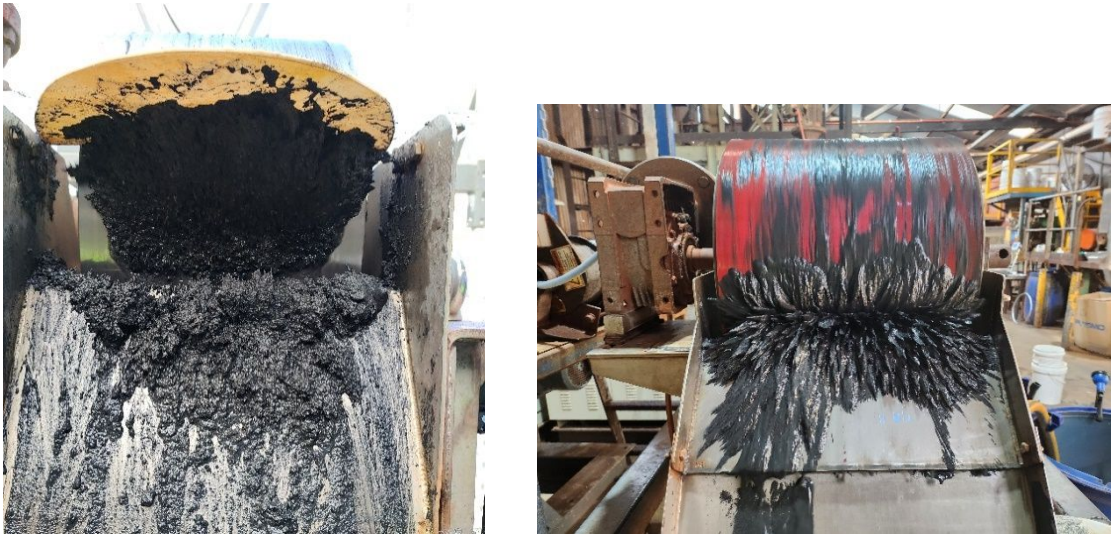
Figure 1 : Bulk MIMS photos showing magnetite concentrate.
