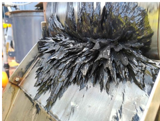
Figure 2 : Bulk LIMS photo showing magnetite concentrate.
