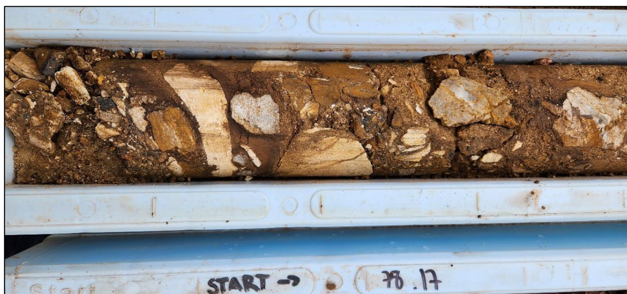
MLJDD020_178.0m_Polymictic Breccia with silica-pyrite clast
