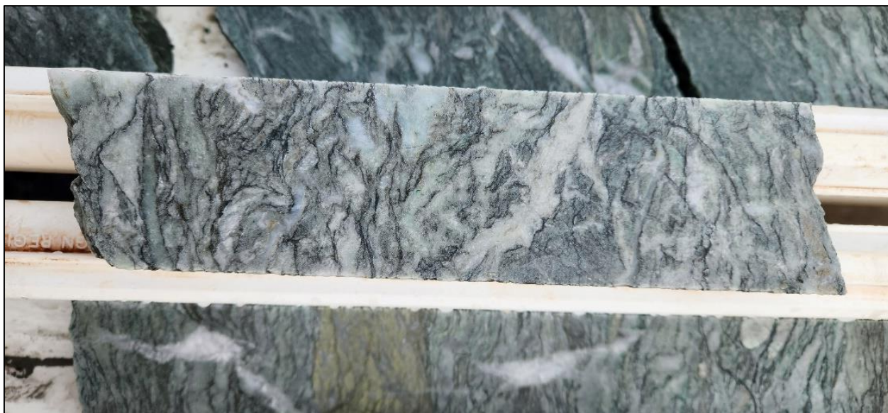
MLJDD019_148.4m_visceral texture in bleached, silicified ultramafic.
