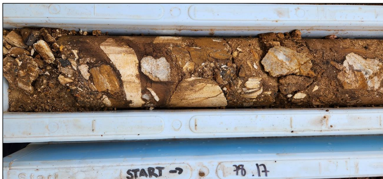
MLJDD020_178.0m_Polymictic Breccia with silica-pyrite clast
