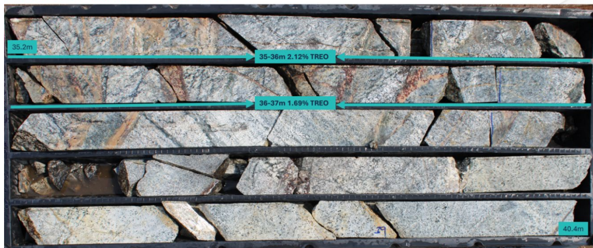
Figure 4. Half drill core of MMD007 showing high-grade rare earth mineralisation in the Machinga deposit.
