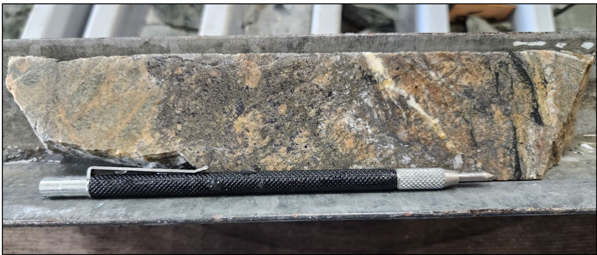
Figure 5: 2019FTD007E, 129.8m - Mineralised carbonate-pyrite-arsenopyrite-cobaltite-scheelite vein (Interval 129.5-130.0m Assay: 0.5m @ 6.64g/t Au, 0.38% Co, 1.02% WO 3 , 0.11% Cu ).
