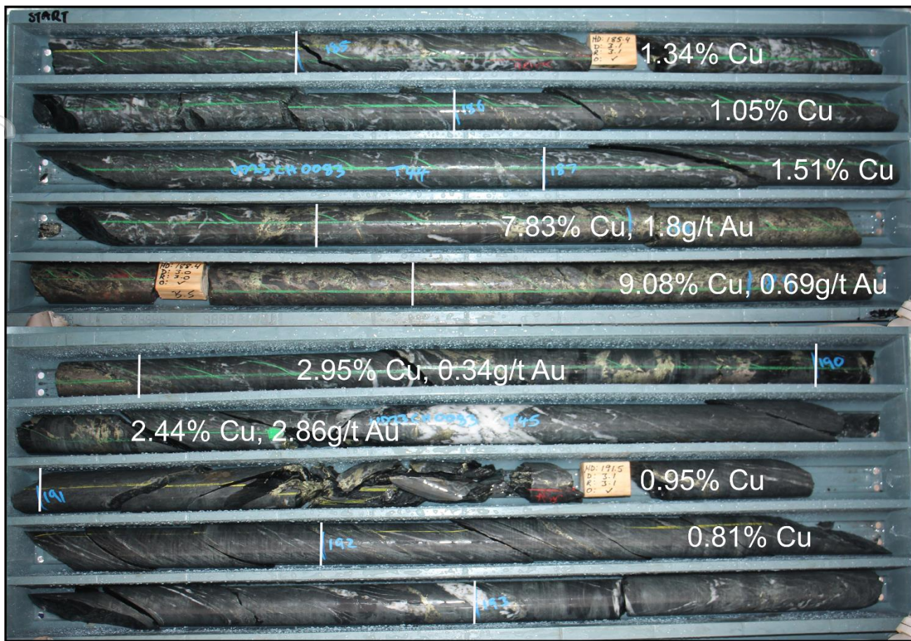
Figure 4. UD23CH0083 drill core photos from 184.6m to 193.6m
