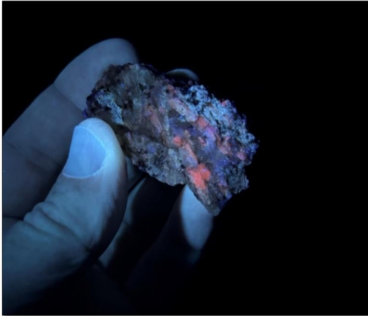
Figure 5: Weathered LCT pegmatite identified from the northern Widgiemooltha project area (UV light 365nm)
