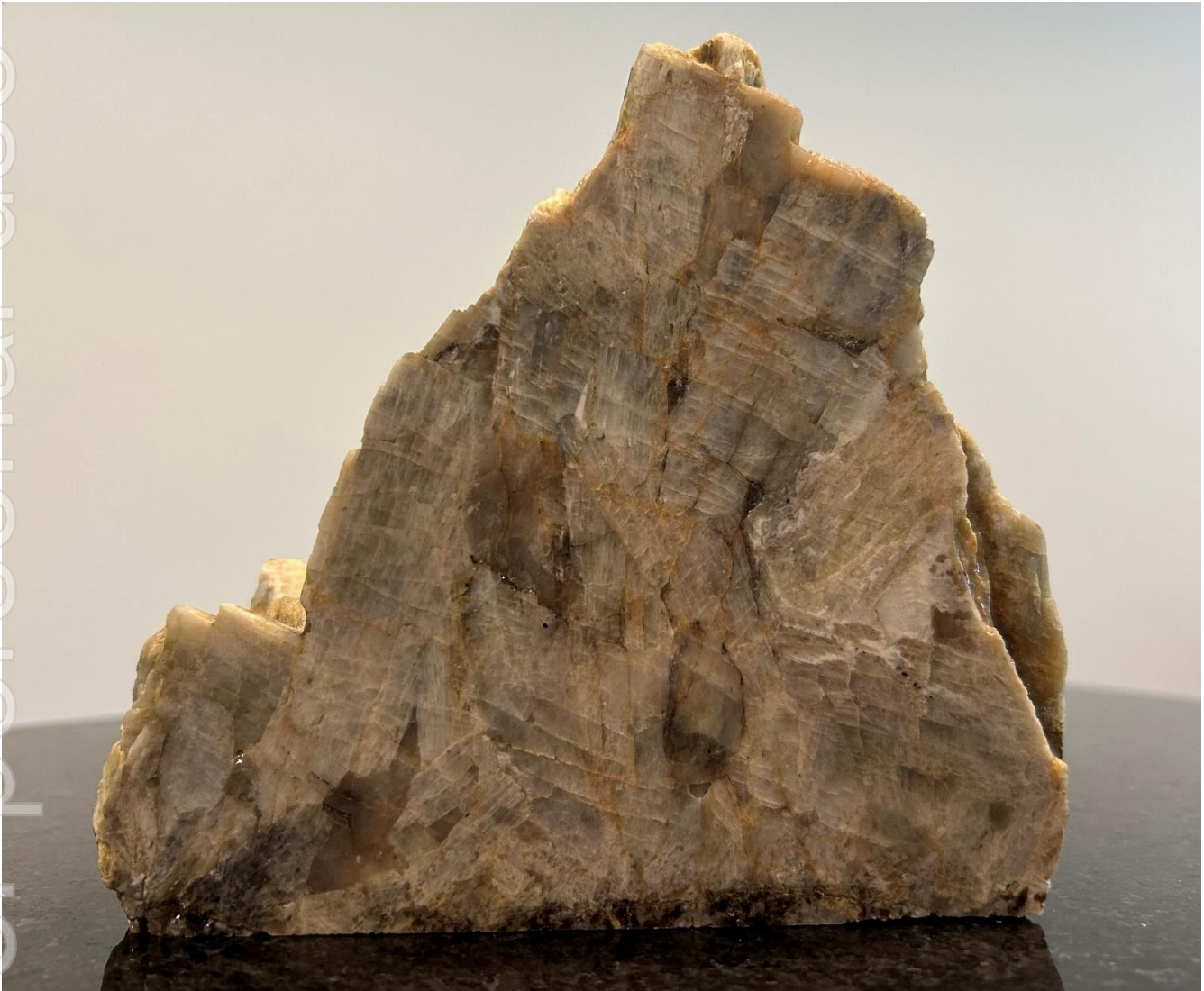
Figure 3: Cut sample of weathered spodumene from the Spargoville Project
