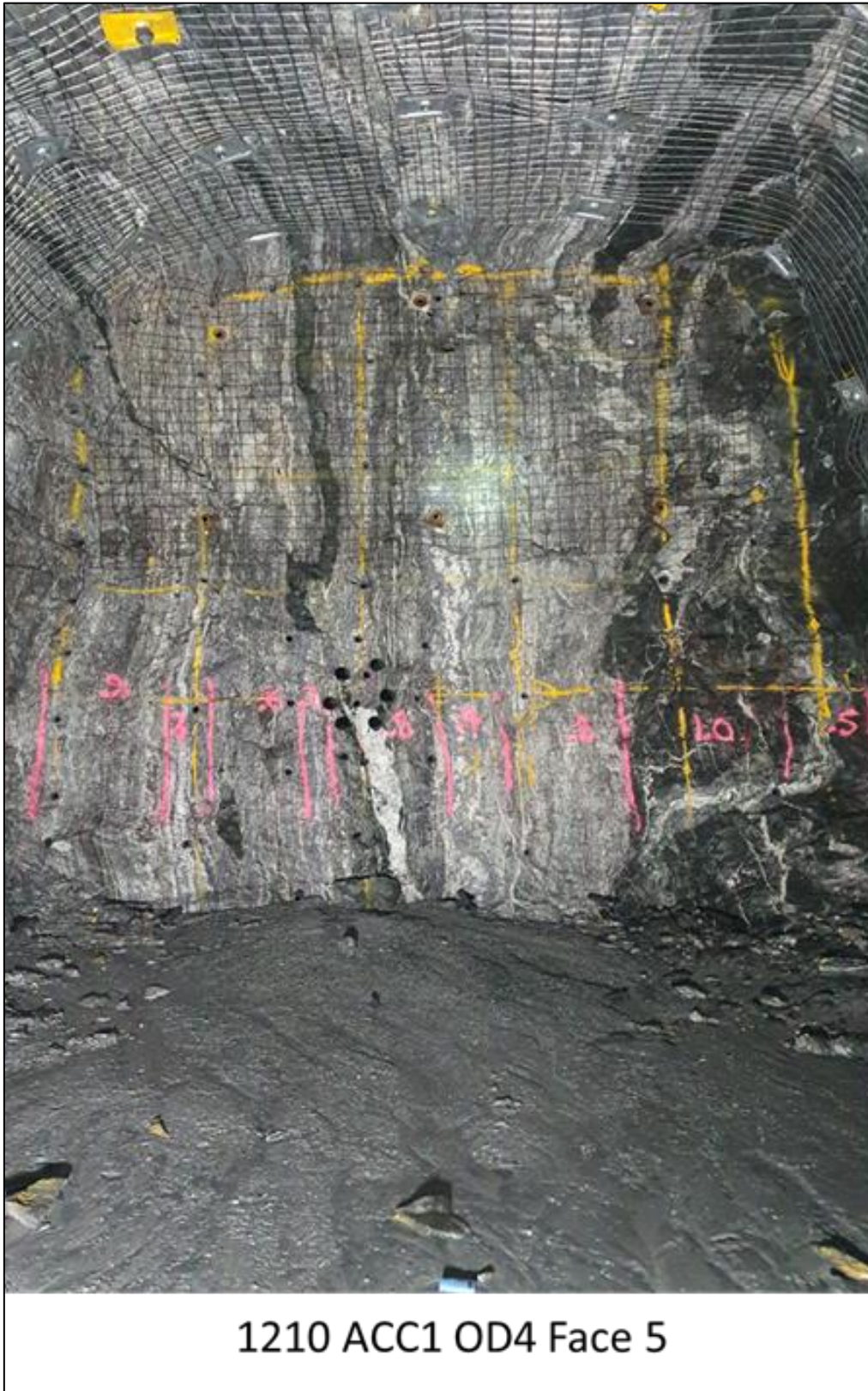
Figure 5 – shows a high-grade core-vein on the newly developed 1210mRL level.
