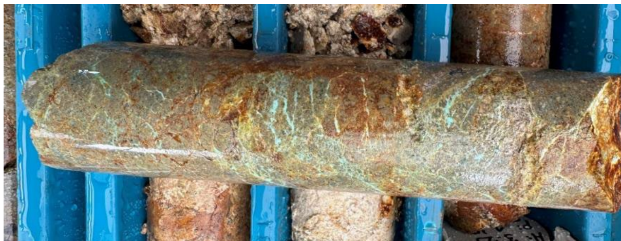
Figure 1: Example of secondary copper mineralisation at around 4-5m depth in 23PCCD0001
