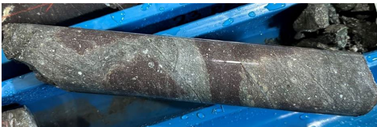
Figure 4: Example of phyllic alteration, quartz – pyrite veins with alteration halo around 429m in 23PFND0001
