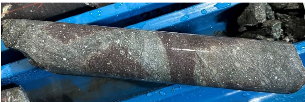
Figure 4: Example of phyllic alteration, quartz – pyrite veins with with alteration halo around 429m in 23PFND0001
