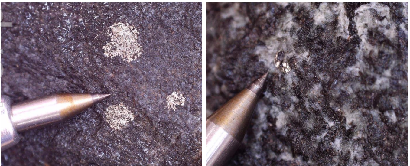
Figure 4. Coarse pyrite in fine-grained chill margin (left) and coarser-grained dolerite/gabbro (right).
