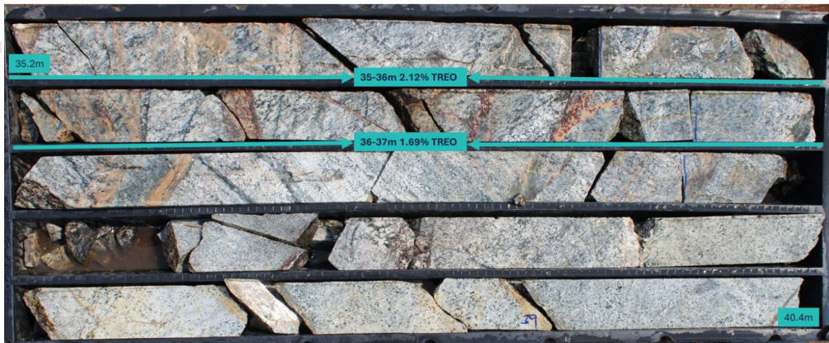
Figure 4. Half drill core of MMD007 showing high-grade rare earth mineralisation in the Machinga deposit.
