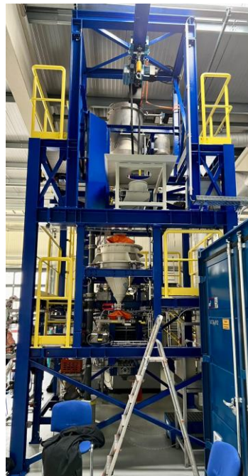
Figure 9 - Pilot Plant calciner and test equipment
