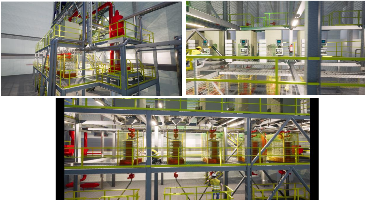
Figure 6 – In-house designed packed bed calciners
