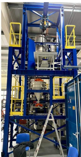
Figure 9 - Pilot Plant calciner and test equipment
