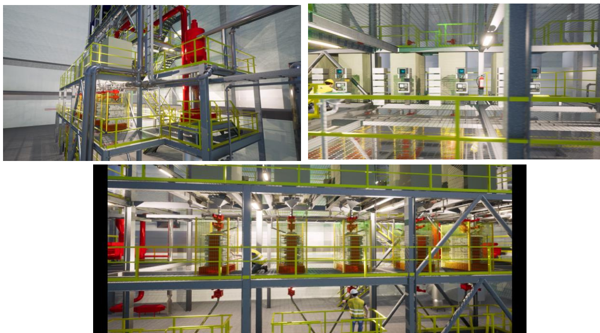
Figure 6 – In-house designed packed bed calciners
