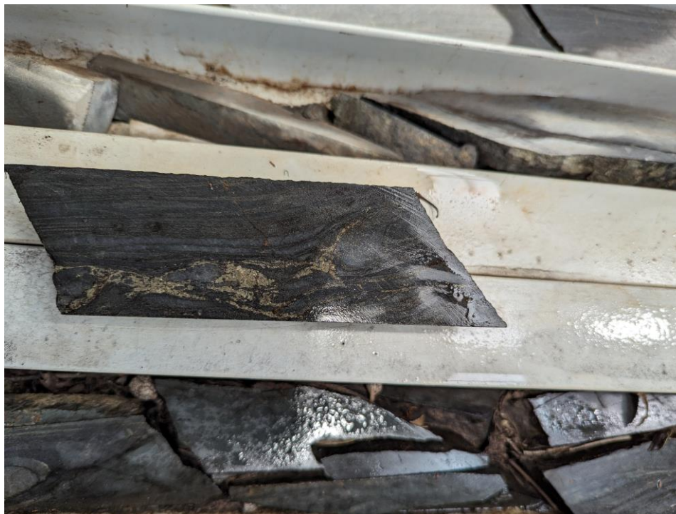
Figure 5. Sulphidised BIF intersected in PMLD9 which originally returned 0.4m @ 1.9g/t Au.
