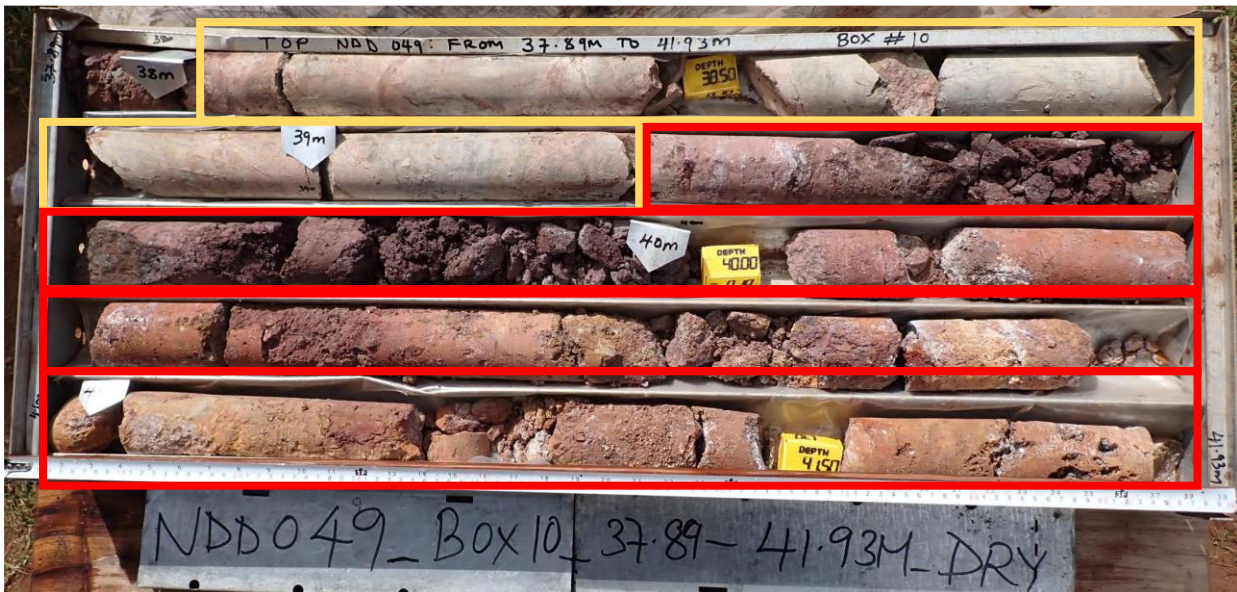
Figure 4. Photos of core from NDD049 (39m to 46m) showing a thick intersection of logged weathered fluorite from 39.3m to 44.5m.
