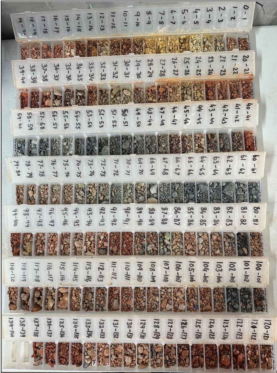
Figure 5. Drill hole HRC23-020 demonstrating propylitic alteration (greenish colour) within metasediments (25m – 75m) overlying microgranite (pinkish red).
