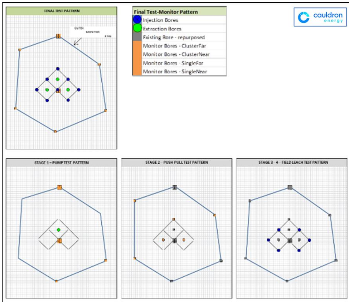
Figure 26: Design of the Proposed Field Leach Trials
