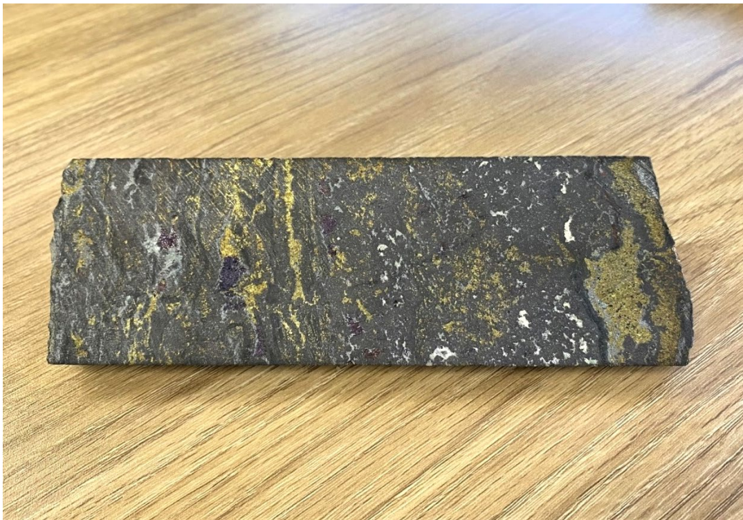
Figure 1: Indium rich chalcopyrite, bornite, and sphalerite in drill core from WD22-01 (interval 543.74-545.11m downhole @ 2.8% Cu, 0.3% Zn, 94.5g/t In, 0.49g/t Au and 39.5g/t Ag). 1
