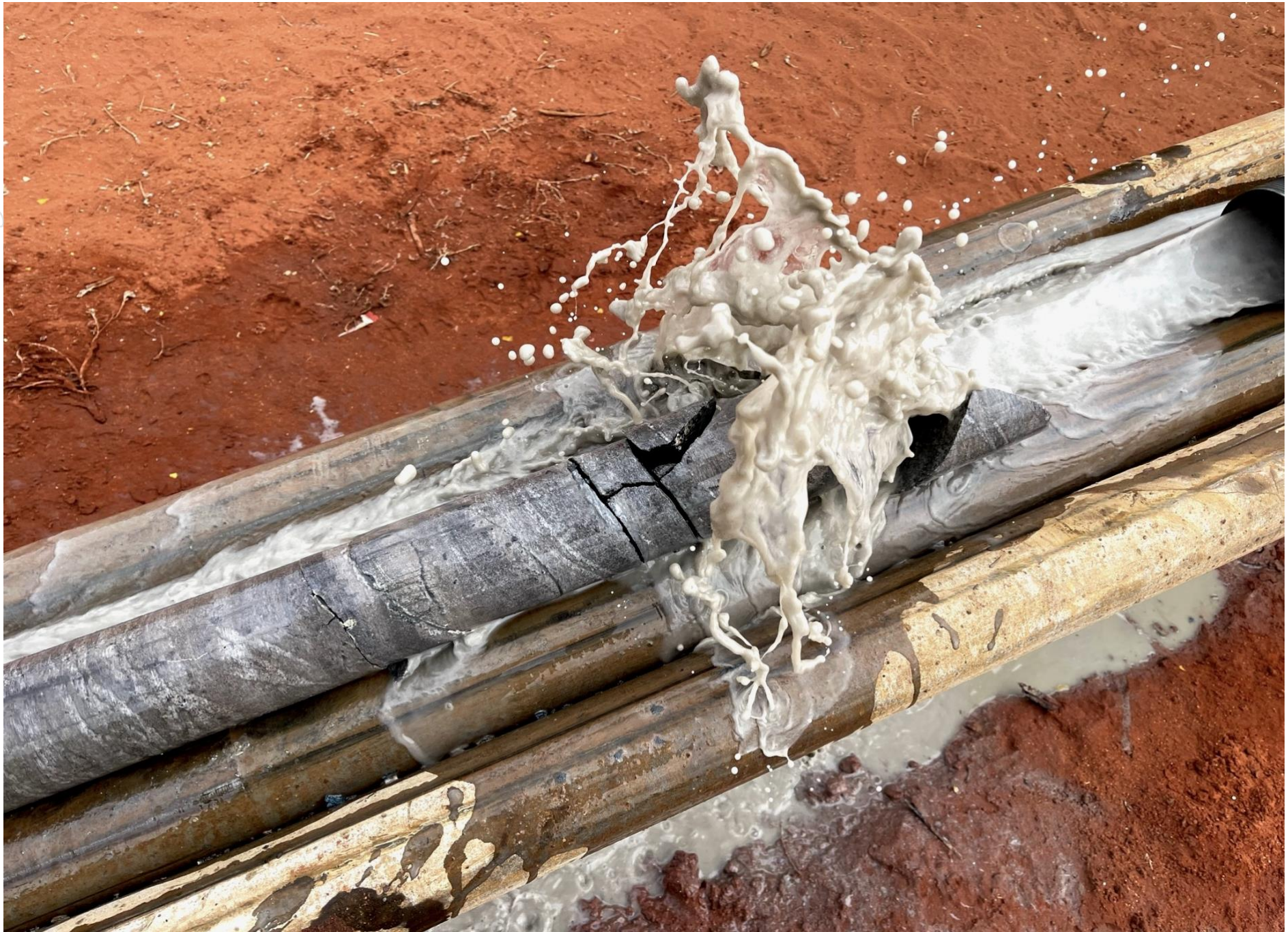
Figure 2: Diamond core being pumped out of the drilling rods at Aurora Tank (May 2023)
