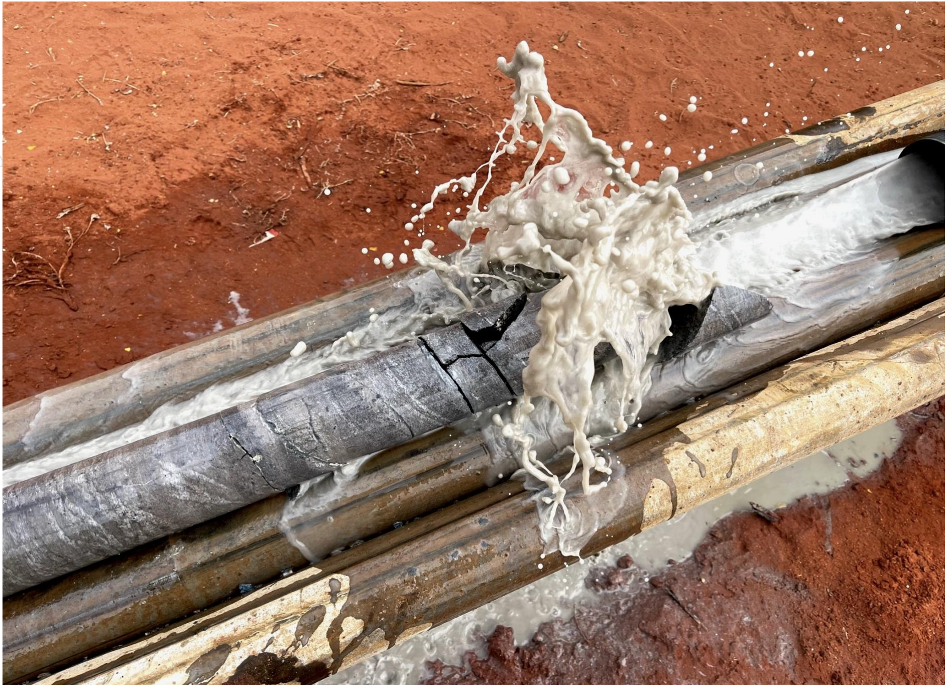
Figure 2: Diamond core being pumped out of the drilling rods at Aurora Tank (May 2023)
