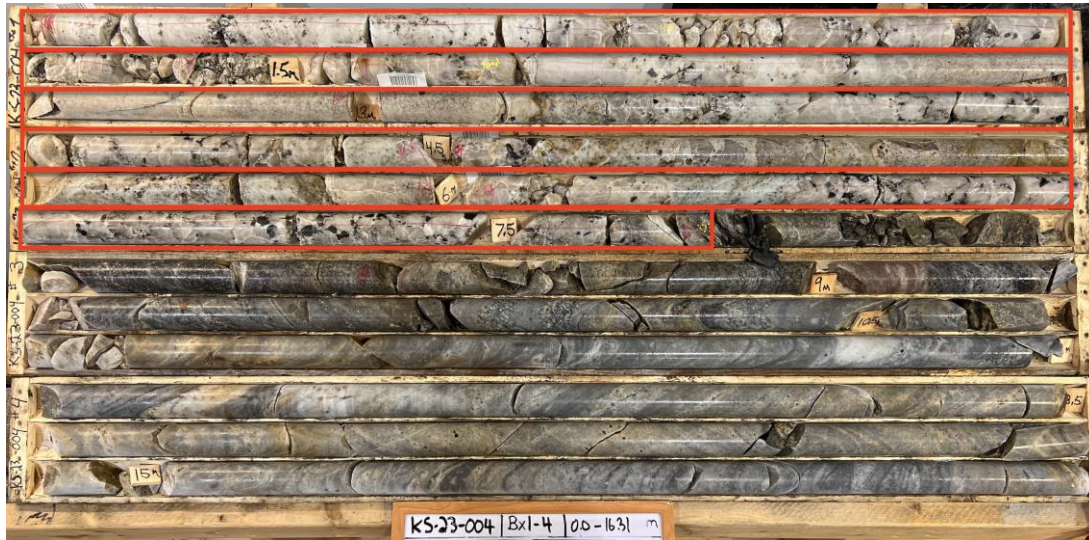
Figure 2 – Core boxes containing spodumene mineralisation in hole KS-23-004
