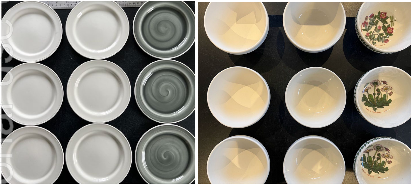
Figure 6: Trial-fired ceramic plates and bowls, manufactured in biscuit (unglazed), glazed and decorated forms (left to right), comprising of trial standard, O/F sample and U/F sample (top to bottom). The trials, which deemed that no visual differences were detected between the trial standard and sample plates, successfully produced industry-accepted standard of ware across all aspects.
