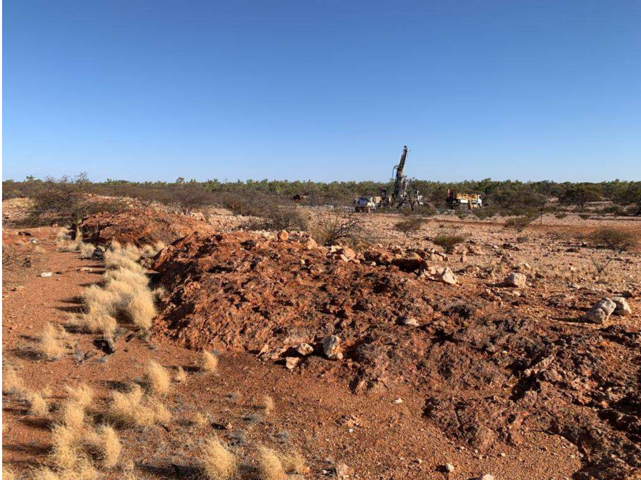
Figure 1: Peggy Sue pegmatite outcrop at the Morrissey Hill Lithium Project, with Strike Drilling RC drill rig at work testing its subsurface continuity.
