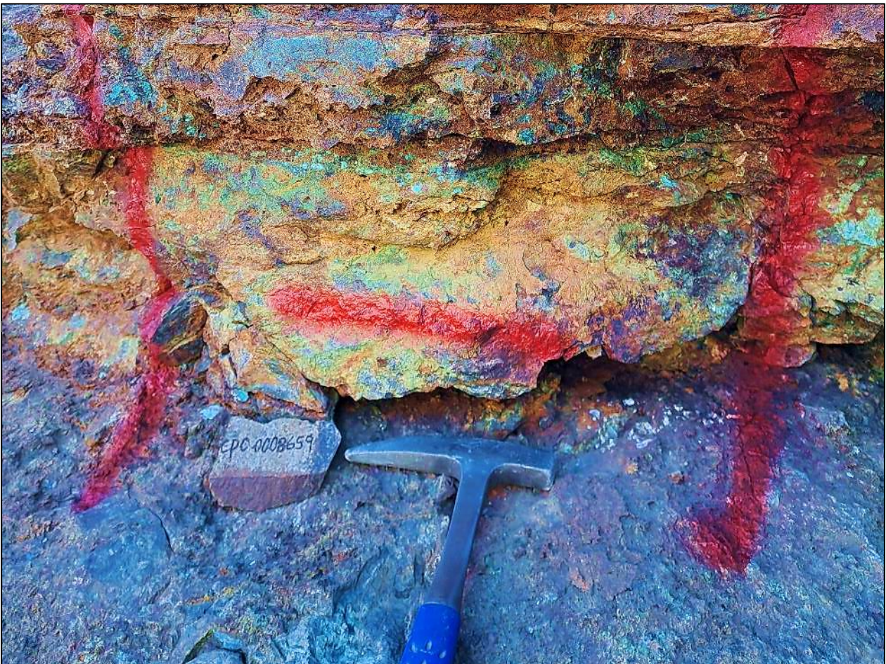
Figure 3: Sample CPO0008659 returned 6.04% Cu and 13.4g/t Au.
