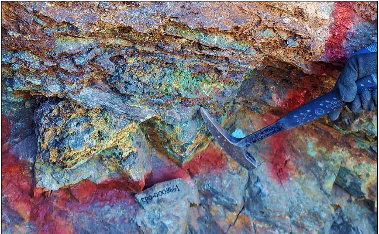
Figure 1: Sample CPO0008661 returned 9.78% Cu and 7.52g/t Au.
