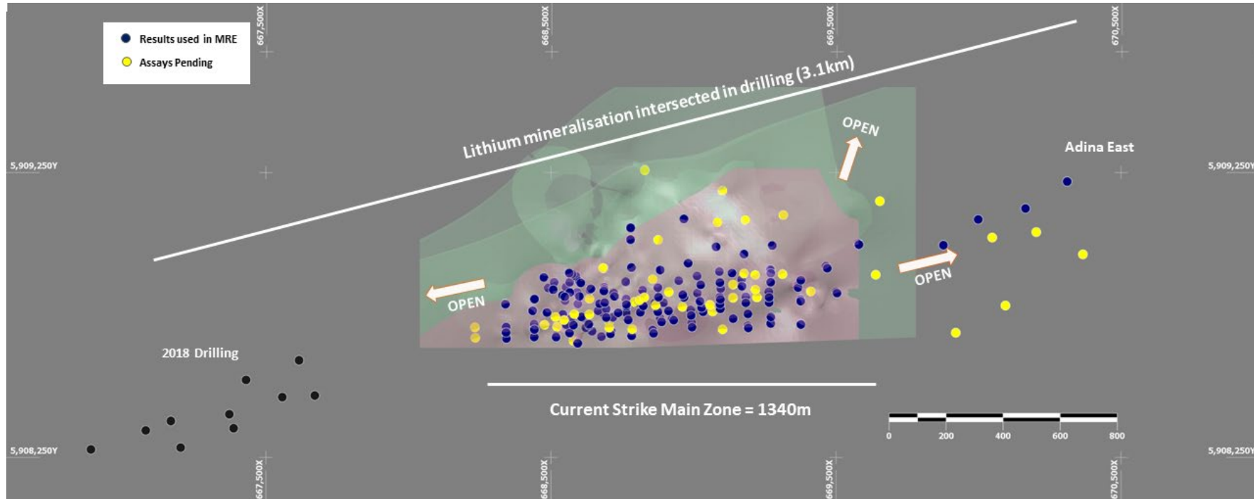
Figure 4: Overview of Adina Prospect showing Mineral Resource wireframes and drilling (including drilling where assays awaited).
