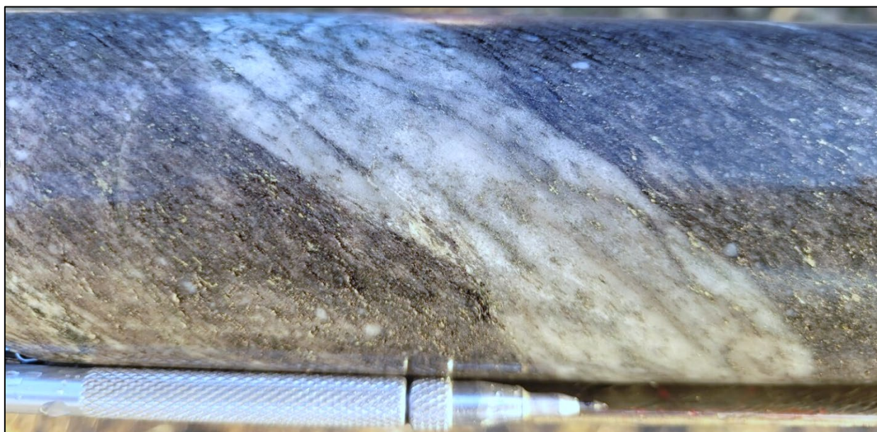
Figure 9. Core from CCDD006 (280.80m) with a 3 cm wide quartz vein with sharp edges and discrete but semi-continuous, wall-rock parallel bands of blebby chalcopyrite-pyrite-pyrrhotite-molybdenite in strongly foliated quartz diorite that has undergone intense potassic alteration by biotite. Such vein textures indicate multiple open-space vein-filling events and extensional “crack-seal” vein growth. These features are characteristic of “B veins” in porphyry copper-gold-molybdenum deposits.
