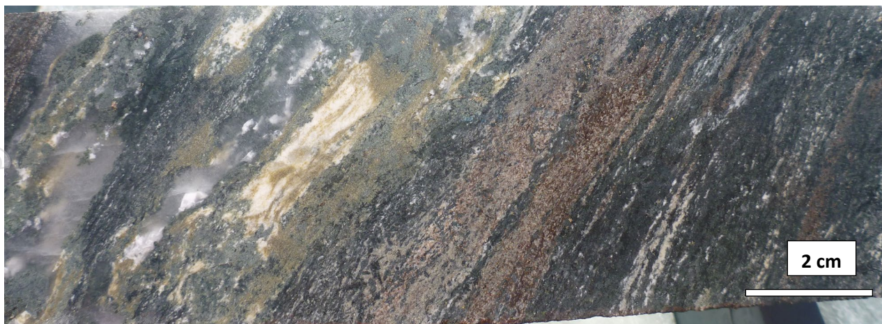
Figure 7. Core from CCDD004 (248.8m). Example of the major alteration types at Cockie Creek. A central 2 cm wide band of pale brown biotite (potassic) alteration in foliated meta-andesite is the earliest stage of hydrothermal alteration. It is replaced by forest green actinolite and greyish white albite (calcic-sodic) alteration that commonly forms selvages around smoky grey quartz veins. The final stage of alteration consists of greenish yellow sericite ± pale green chlorite ± pistachio green epidote ± milky white carbonate. Pyrite-chalcopyrite ± pyrrhotite ± molybdenite mineralisation commonly accompanies potassic and (calcic-sodic) alteration. Alteration is preferentially focussed along pre-existing foliations.
