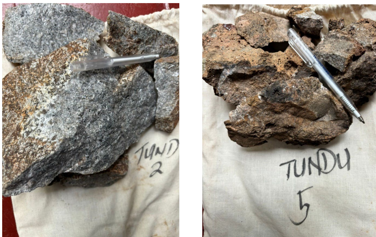
Figure 4. Rock chip samples 2 and 5 from Tundulu, left: visible syenite and right: visible brecciated carbonatite
