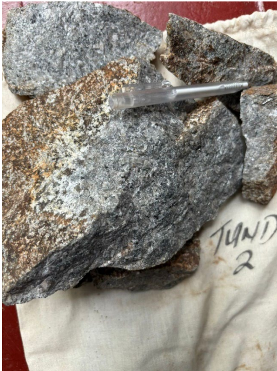
Figure 4. Rock chip samples 2 and 5 from Tundulu, left: visible syenite and right: visible brecciated carbonatite
