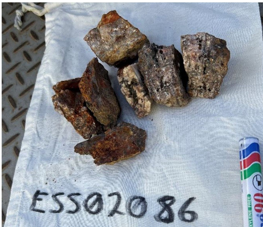
Figure 2 - Breccia vein sample from Sandy Creek area returning 36.1ppm Au and elevated pathfinders Cu, Pb, Zn, As, and Cd (see ESS02086 location coordinates 768480E/ 7974337N plotted on Figure 1)
