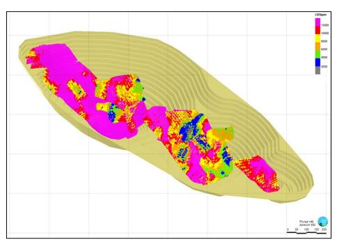
Figure 11: Oblique view Root Bay Block Model and pit design
