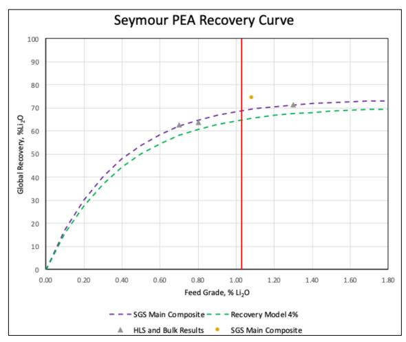
Figure 8: HLS Test Results (Purple curve) with Seymour Predicted Recovery (Green curve)
