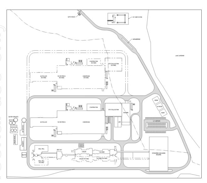
Figure 35: Lithium Hydroxide Conversion Plant Layout
