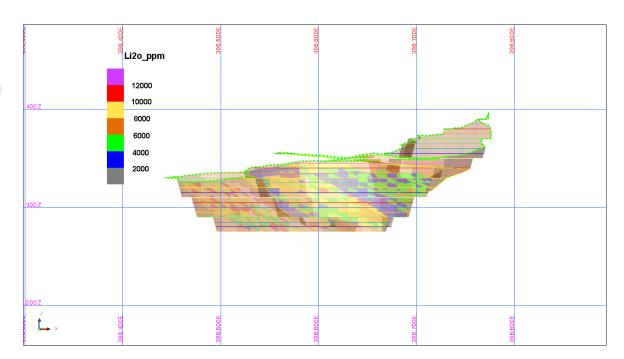
Figure 17: Section View Proposed Pit Design - South Aubry
