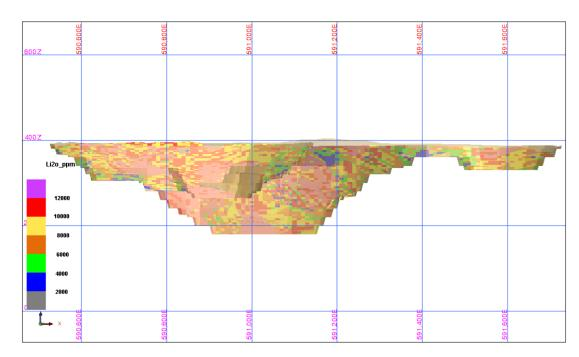
Figure 23: Section View of Proposed Pit Design - McCombe
