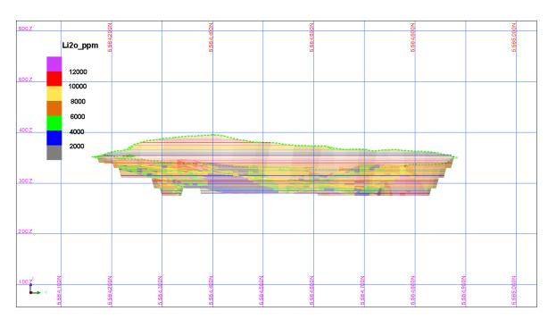
Figure 18: Long Section of Proposed Pit Design - South Aubry
