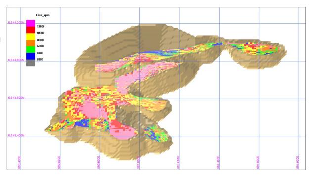
Figure 12: Oblique view McCombe Block Model and pit design
