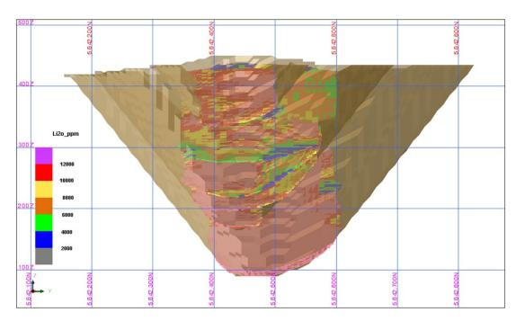
Figure 21: Long Section View of Proposed Pit Shell for Root Bay
