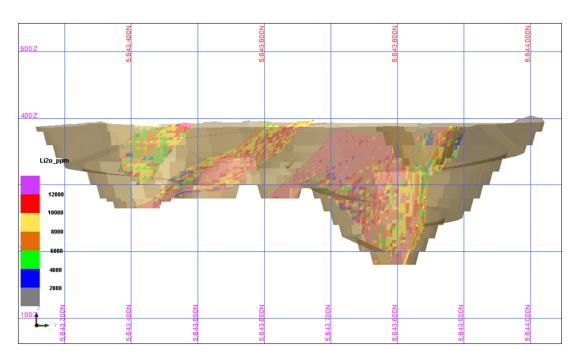
Figure 24: Long Section View of Proposed Pit Design - McCombe
