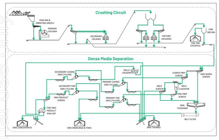
Figure 28: Seymour Project (Stage 1) Simplified Concentrator Flow Sheet
