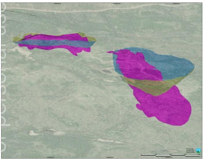
Figure 3: Aubry Interpreted Pegmatites with Overlayed Pit Designs
