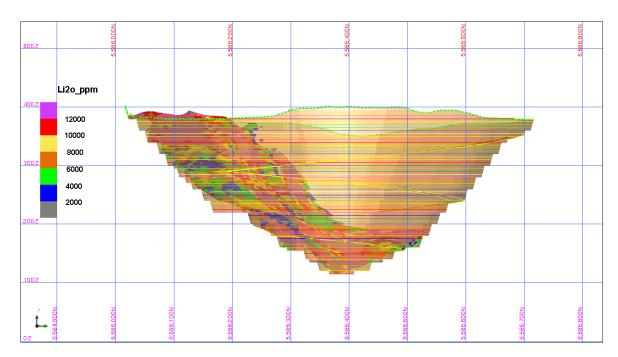
Figure 15: Long Section View of Proposed Pit Design - North Aubry
