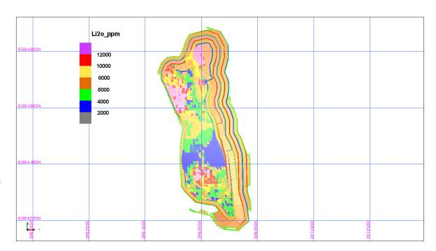
Figure 16: Plan View of Proposed Pit Design - South Aubry
