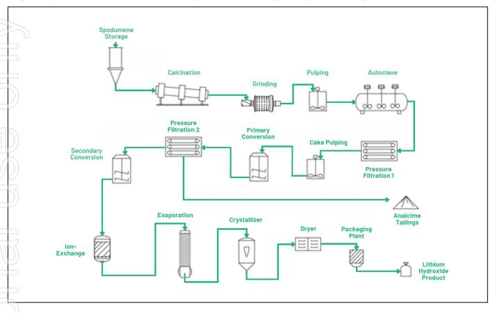
Figure 29: Simplified Lithium Hydroxide Conversion Plant Flowsheet (Carbonation Leach)
