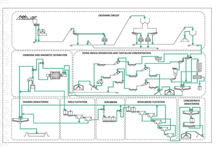
Figure 30: Root Project (Stage 3) Simplified Concentrator Flow Sheet
