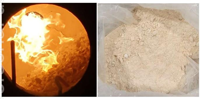
Figure 9: Rotary kiln start (LHS) and end (RHS) bulk calcination test Comp 2
