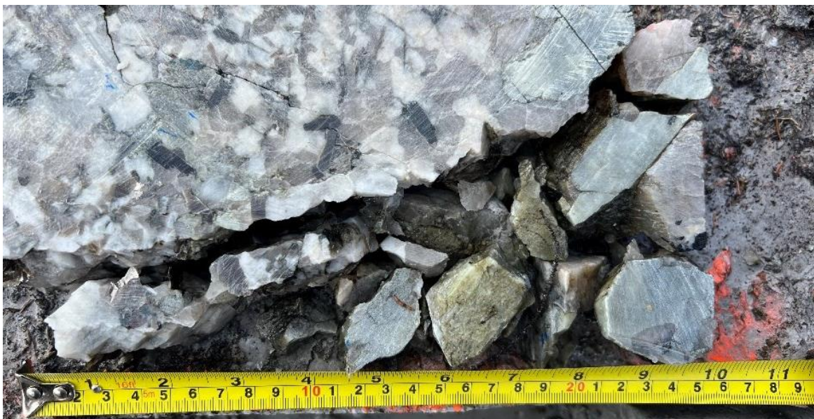
Figure 4: Spodumene Bearing Pegmatite from Channel Sampling
