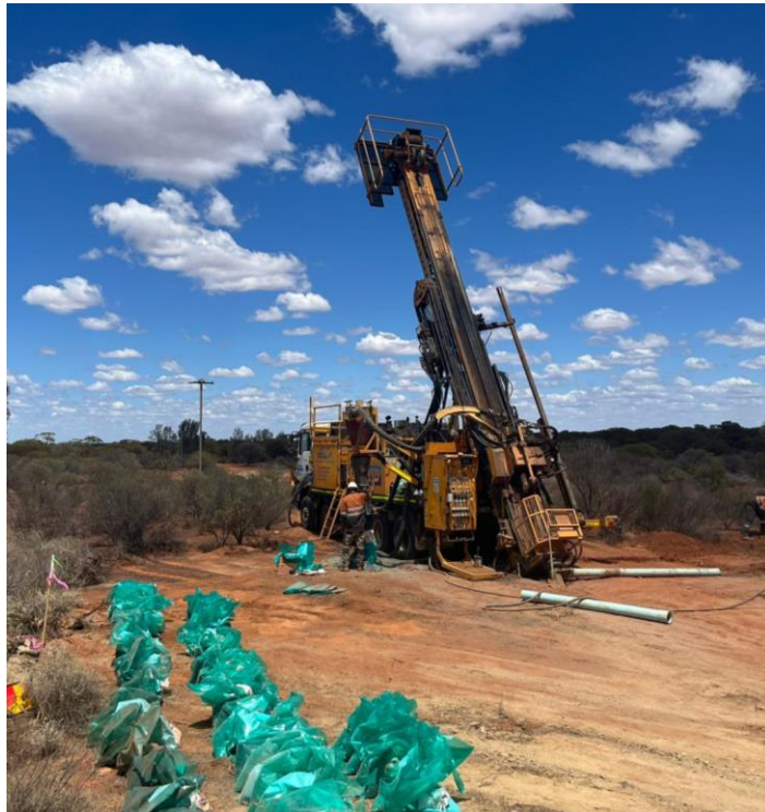
Figure 6 - Reverse Circulation Drilling at Menzies (Aspacia)
