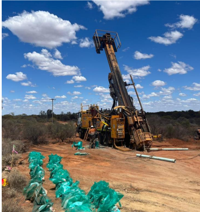
Figure 6 - Reverse Circulation Drilling at Menzies (Aspacia)
