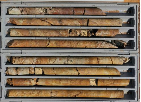
Trays 9 and 10 of diamond drill hole 23YJDD219 between 28.35 and 35.06 m depth. Veining and structural deformation have been logged throughout the entire section (see Appendix B for details).
