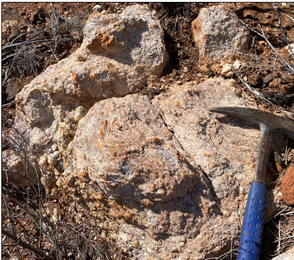
Photograph 1. Pegmatite outcrop containing spodumene crystals (rectangular pale grey; visually estimated at 40-50 vol%) in a strong shear foliation; assayed at 4.19% Li 2 O.
