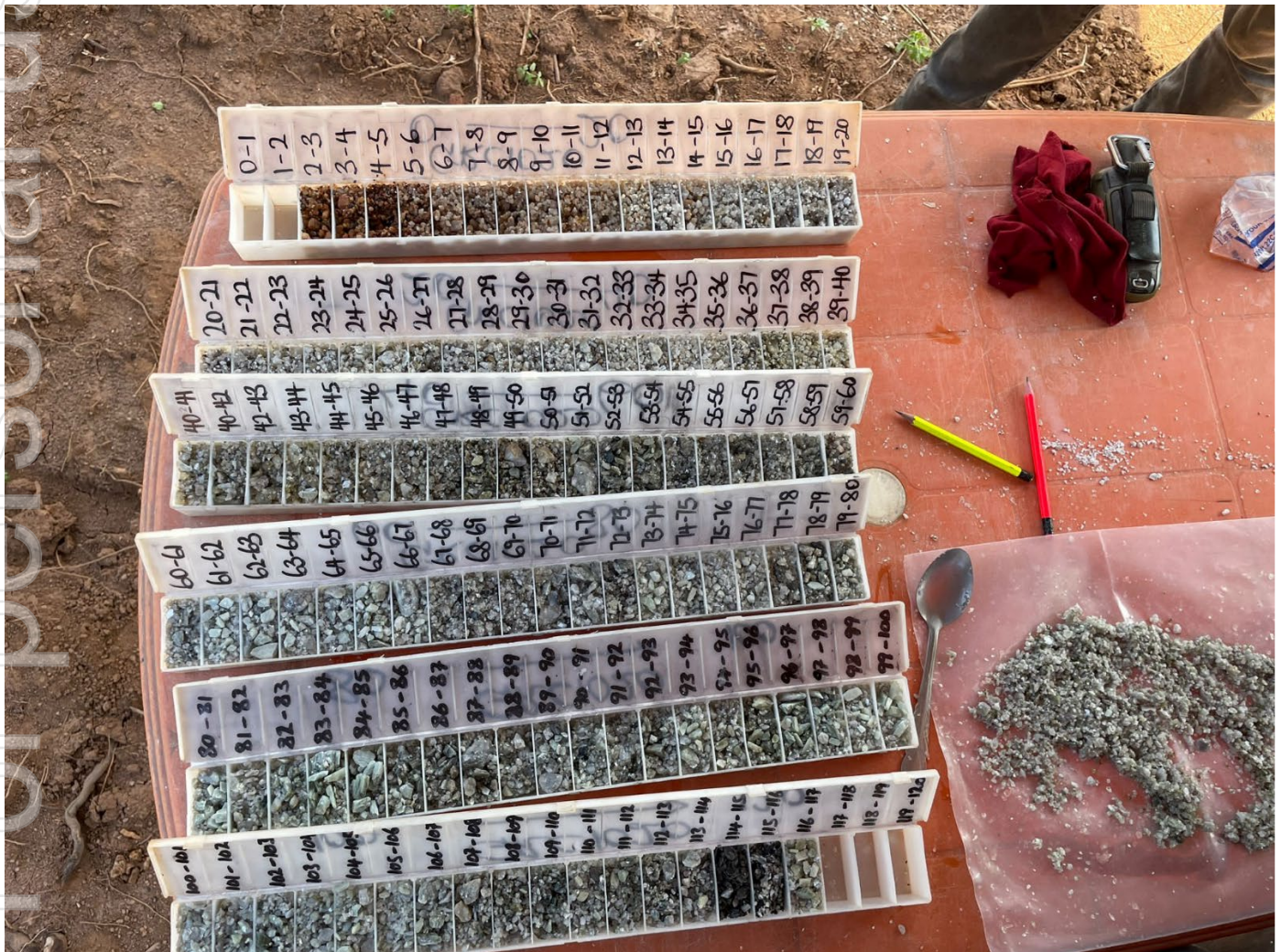
Figure 1: 106m continuous pegmatite interval from 6m observed in hole GRC1020 with coarse fragments of visible spodumene evident. Further pegmatite with coarse-grained visible spodumene intersected from 116m to 122m and 137m to 178m with end of hole at 250m (not shown in this photo)
