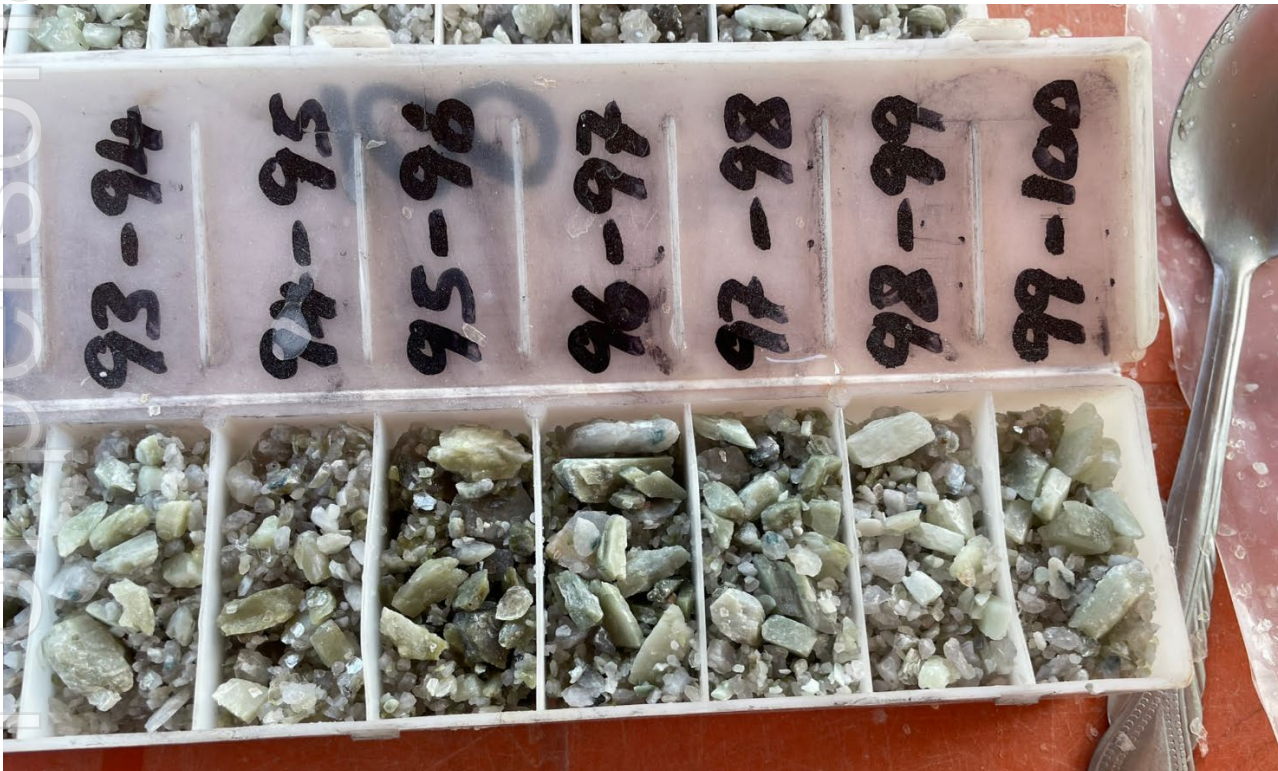
Figure 3: An example of the coarse fragments of visible spodumene in RC drill chips logged in hole GRC1020 with meter depth intervals marked
