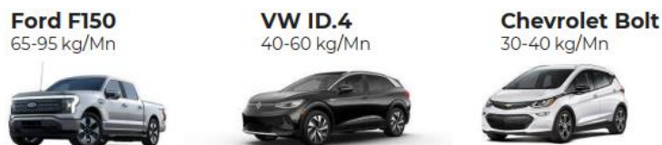
Figure 5: Manganese content (kg) in per battery in each vehicle above (Source: Benchmark Mineral Intelligence)
