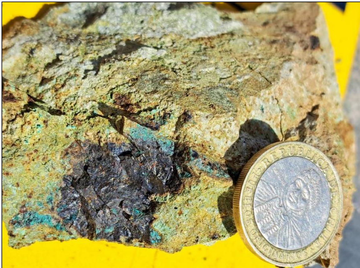
Figure 3: Significant copper (malachite, bornite and chalcopyrite) mapped in outcrop, sample number
