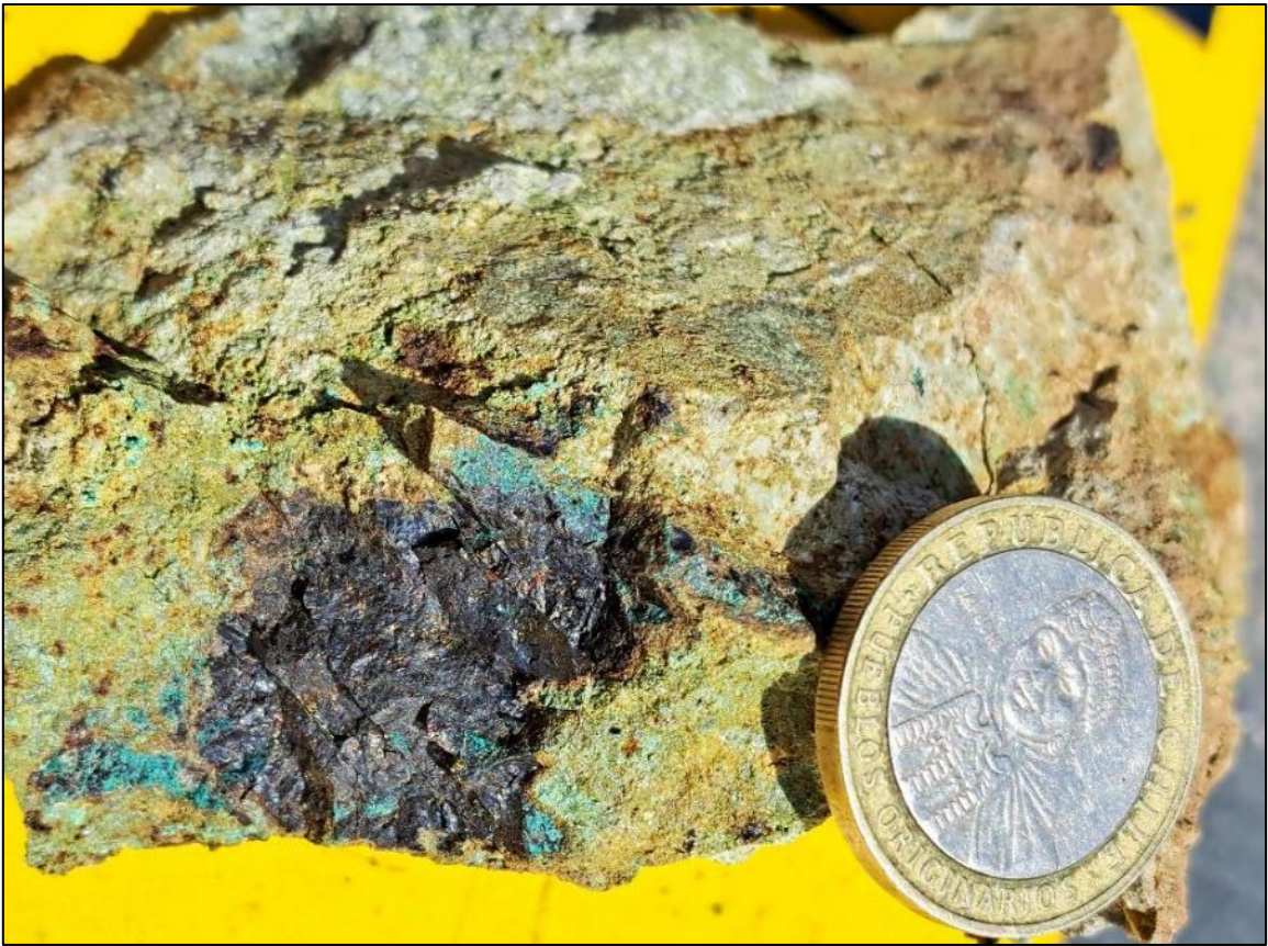
Figure 3: Significant copper (malachite, bornite and chalcopyrite) mapped in outcrop, sample number CPO0008615, returned 5.37% Cu.
