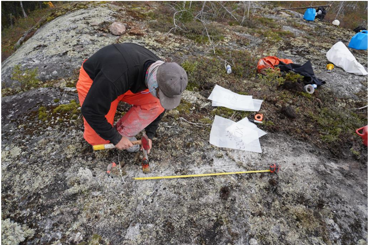
Photo 3: Pegmatite* at Monaro north project area - rock-saw cut lines and cut channel sampling in progress
