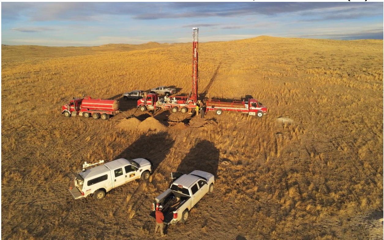
FIGURE 1. MUD ROTARY DRILLING AT GTI'S LO HERMA PROJERCT, POWDER RIVER BASIN (WY)
