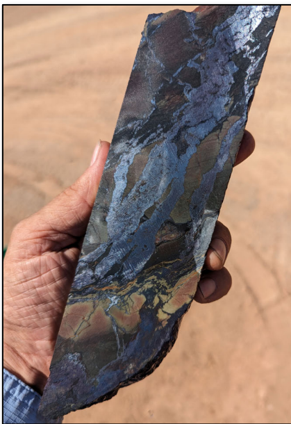
Figure 3. Strong chalcocite (silver grey to black mineral) vein and vein breccia mineralisation in MOXD225 from interval 0.70m @ 26.90% Cu, 225g/t Ag & 78 ppm Co from 352.5m downhole.
