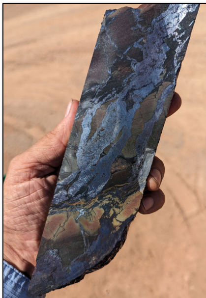
Figure 3. Strong chalcocite (silver grey to black mineral) vein and vein breccia mineralisation in MOXD225 from interval 0.70m @ 26.90% Cu, 225g/t Ag & 78 ppm Co from 352.5m downhole.
