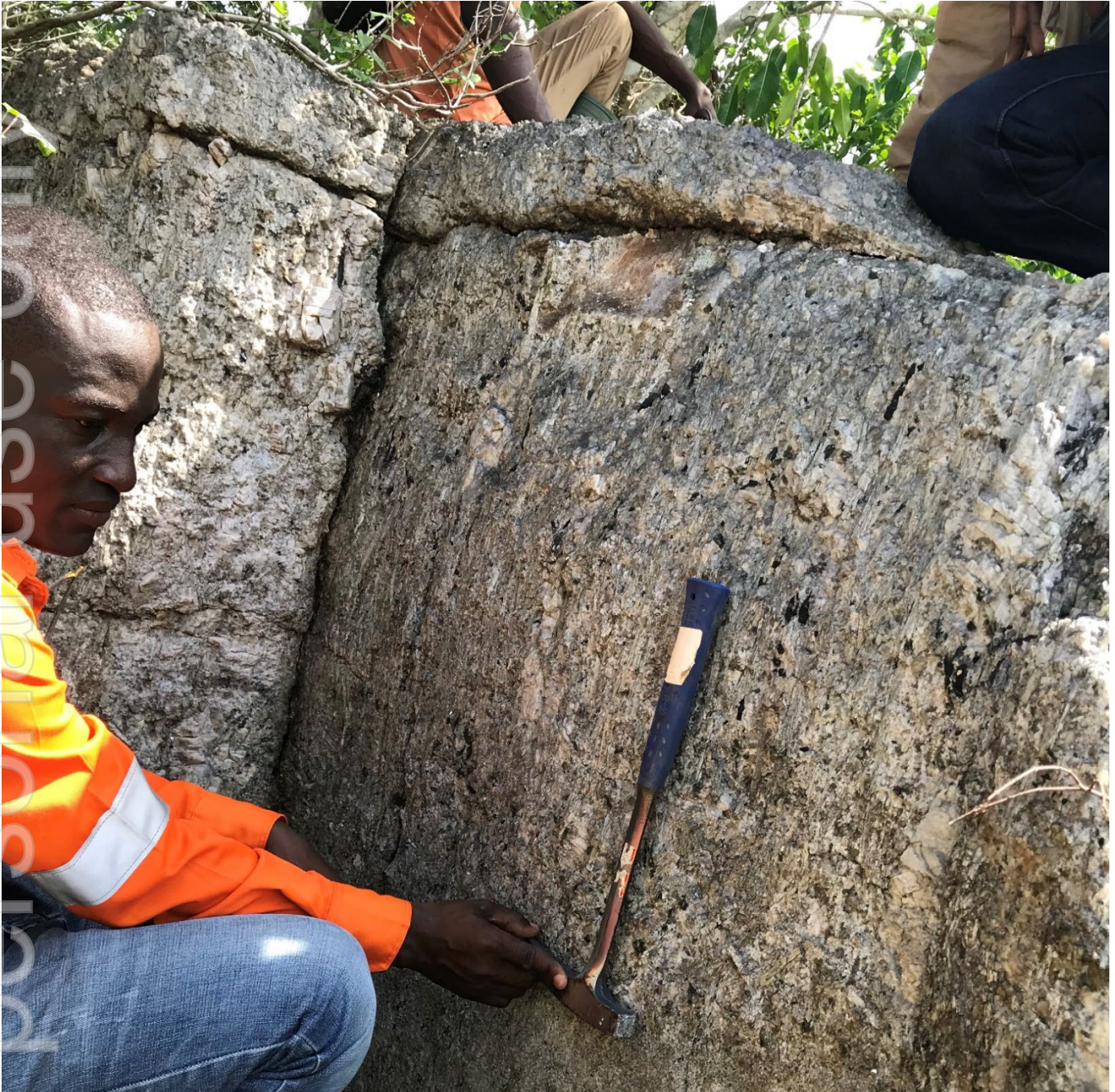
Figure 4: Spodumene-rich pegmatite outcrop on Egyasimanku Hill with spodumene crystals (green) evident parallel to the direction of hammer handle throughout the outcrop.
