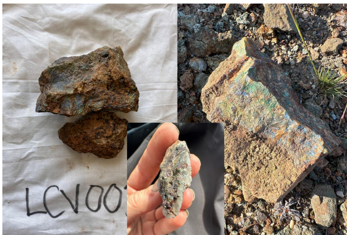
Figure 2. Copper minerals including bornite, chalcopyrite, azurite and malachite from Long Tunnel Prospect.
