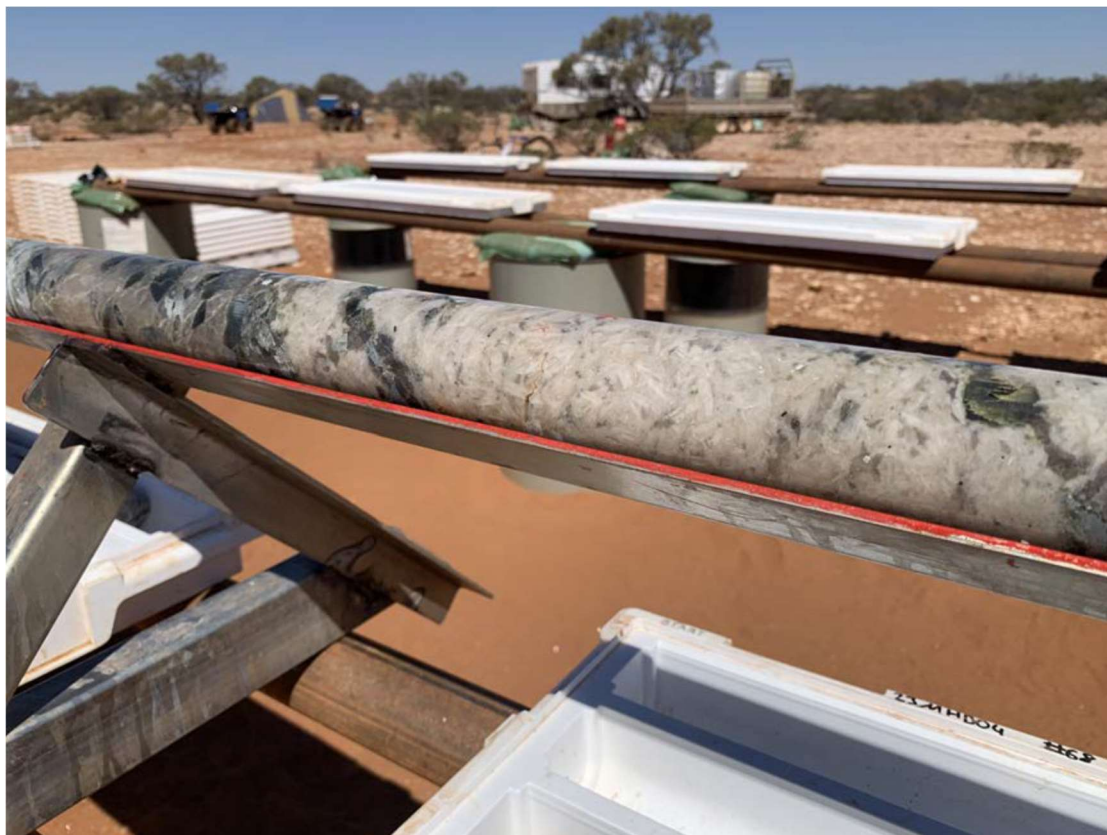
Figure 1: Pegmatite drill core from the Morrissey Hill Lithium Project Phase 1 drill program Hole 23MHD003: 3.9m @ 0.2% Li 2 O from 74.8m downhole depth.
