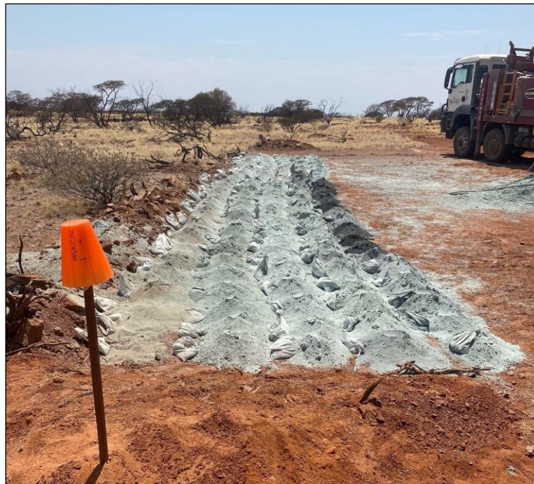
Figure 2. Hole MSCR012 – showing black RC piles containing copper sulphides.
