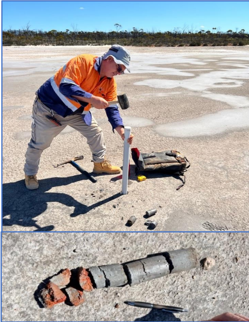
Figure 4. Lake Hope showing the push tube sampling method (!) and an example of the lake clay from the push tube.
