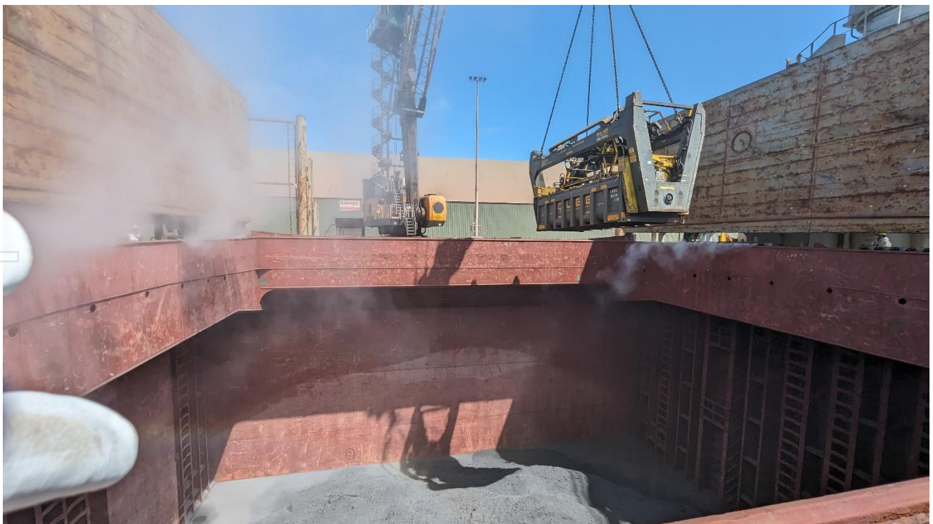
Figure 2 – Qube Logistics Services transferring the Rotabox™ containers to the ship for unloading. Once inside the ship’s hold, the lifting mechanism rotates the container to place the concentrate in the hold (photo 7 November 2023).
