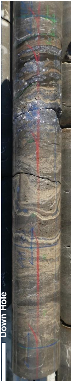
Figure 4: Close up photograph of drill core interval 245.3m to 246.1m showing colloform massive sulphides (low-iron sphalerite = cream coloured & galena = blue grey).
